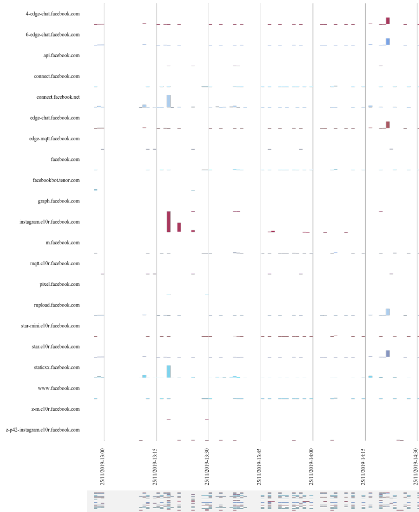
Figure 5.13: Data flow to IPs received by different DNS host names (Y-axis) that match the user specified regular expression for Facebook over time (X-axis)
