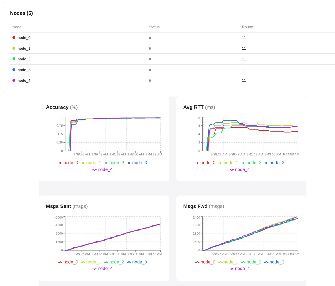
Figure 5.7: The node table and the metric charts below stream live values over server-sent events once the run is underway.
